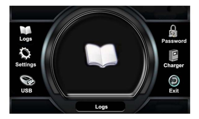
When the charger is idle, press and hold <ESC>, the Main Menu is then displayed. The main menu is automatically exited after 60 seconds of inactivity or can be exited voluntarily by pressing the <ESC> button.
