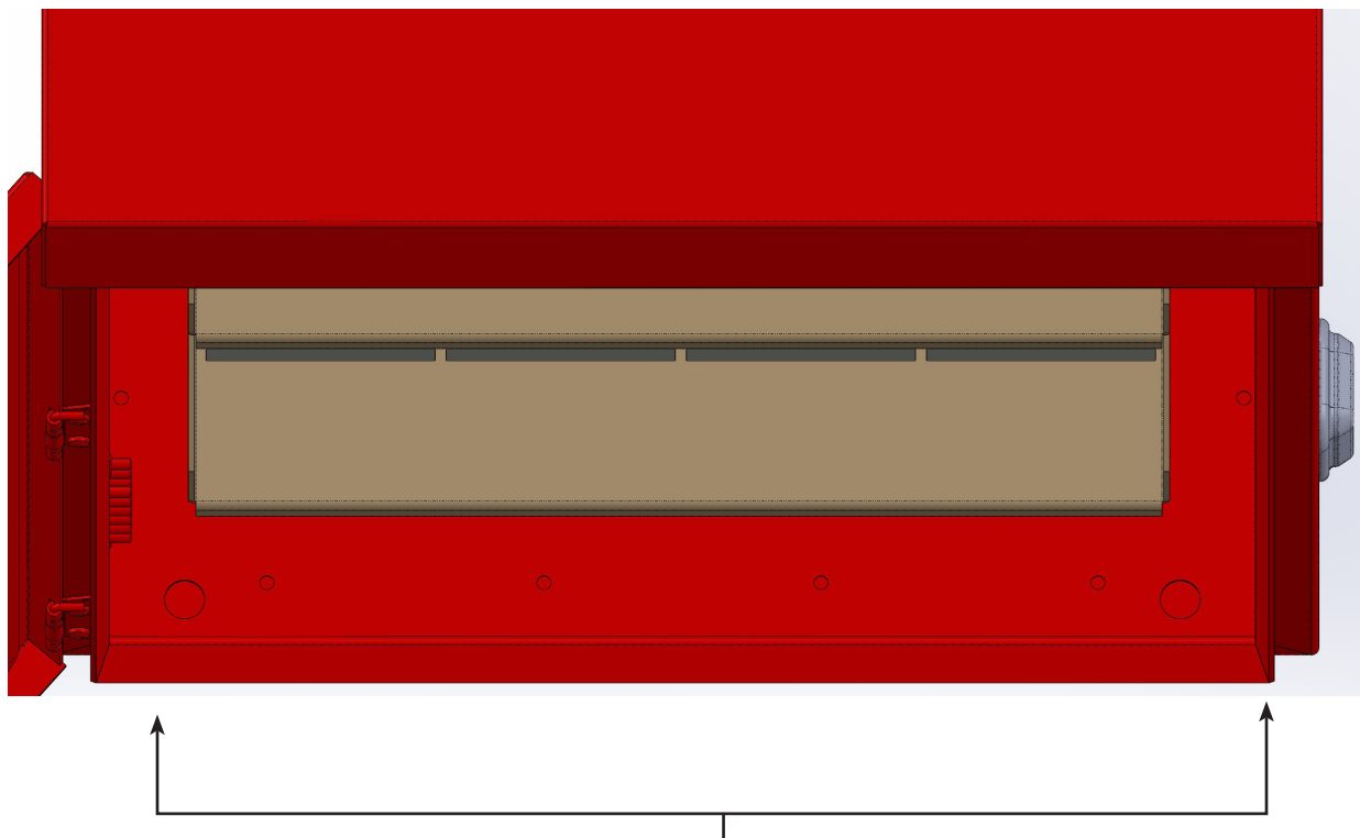
Four of the 16 mounting holes around the base of the enclosure
