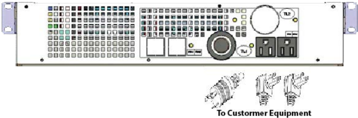
Two twist lock Receptacles in PDU Extension, Dual phase AC out connections
