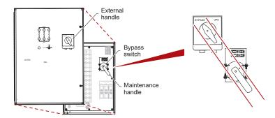
2. If the two handles are not aligned when the door is closed, turn the outside handle until it engages with the maintenance handle. **Note**: You will hear a **clicking** sound with the two handles engage.
