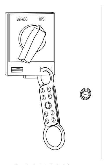
Figure 2 — Lockout with a Padlock
