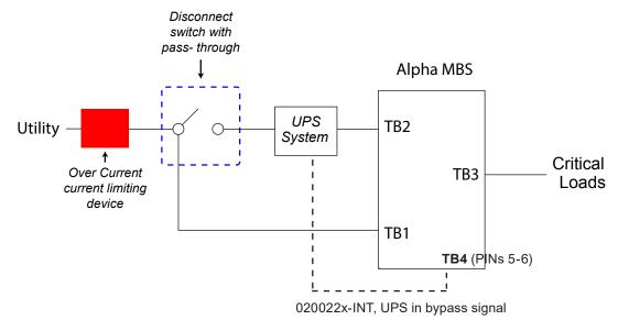
Figure 7 — Typical MBS Wiring Diagrams
