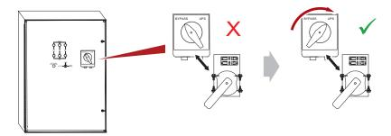
3. To prevent the outside maintenance handle from moving, lock it into position with a padlock.
