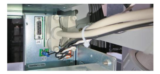
3.6. Route only the 2x DB-25 cables in to the distribution. Do not move or remove any other wires from the interface PCBA (Item 1).
