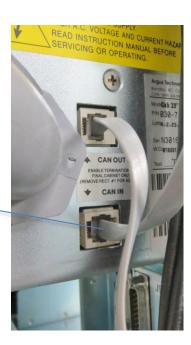
1.8. Route the 2x DB-25 cables and the CAN cable in to distribution. Do not remove any cables or wires from the CXCM4 interface PCB.
