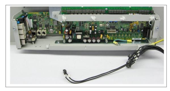
5.4. Remove the CXCP from the door on the Vista power system. (save the hardware to mount the CXC-HP assembly).
