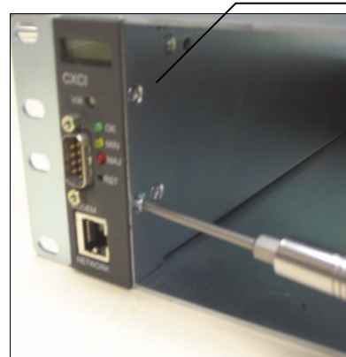
Figure 8—Showing CXCI module installation
