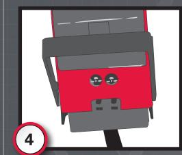
Make sure the battery and charger connectors are fully connected.
