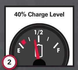
To maximize battery life, batteries should not fall below 40% charge level.
