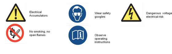
Labelling may vary due to application and dimension of the Battery. The manufacturer, respectively the importer of the batteries shall be responsible for placing the symbols (a minimum size is specified). In addition, consumer/user information on the significance of the symbols may be attached.
